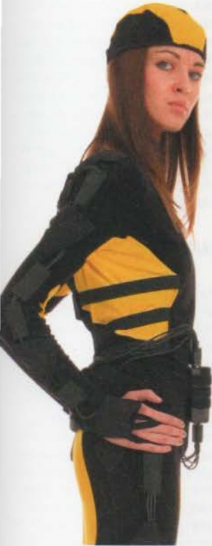
Animazoo's GypsyGyro-18 motion-capture suit contains 18 gyroscopes which transmit positional and rotation data wirelessly to a base station. As well as providing clean data, the system can capture multiple actors in realtime
